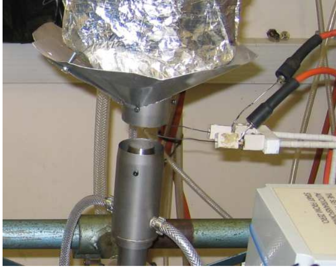
Figure 2.4: Photograph of the counter-flow test rig with spark electrodes.
