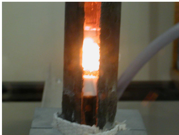
Figure 3.2: Methanol flame stabilized at ceramic's interface.
