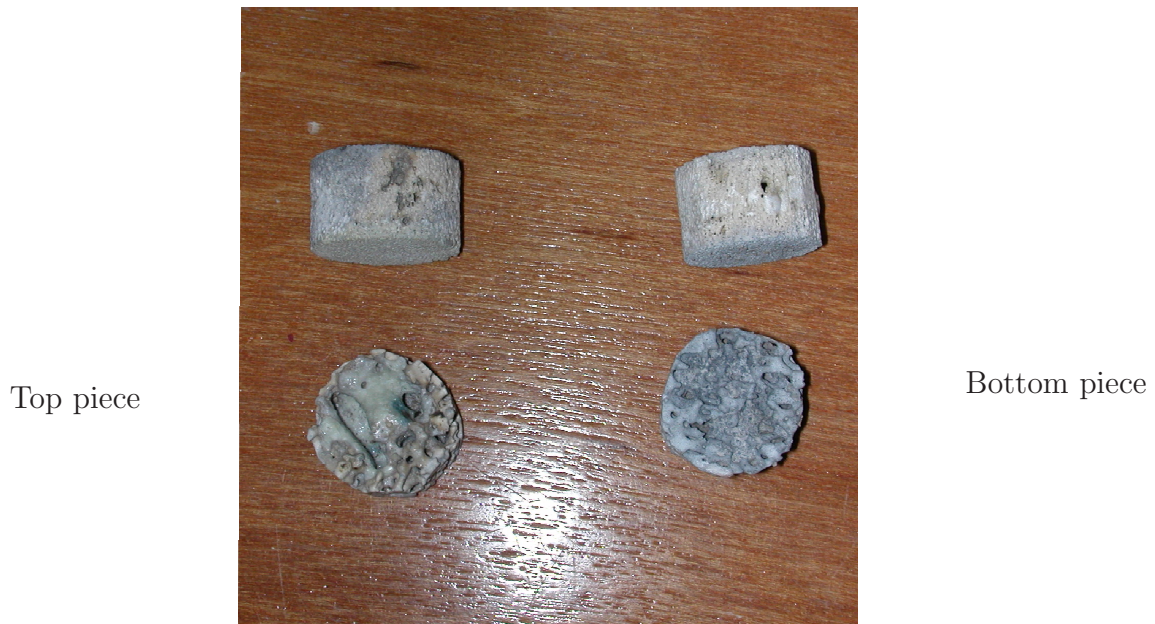
Figure 3.3: Damaged pieces of cordierite.
