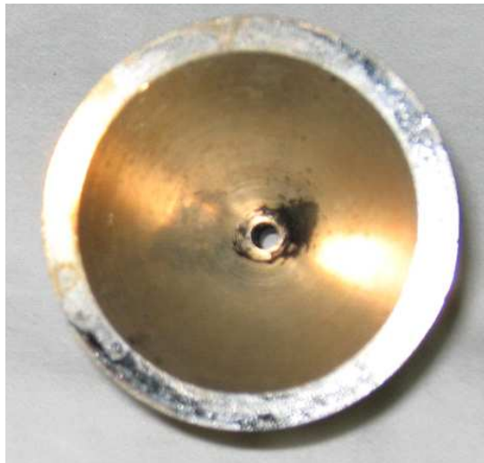
Figure 4.5: Adapter to burner after lean acetylene/oxygen flame.
