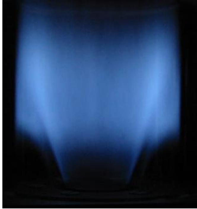
Figure 2.11: Photograph of an unforced fully premixed flame. Conditions are: \langle U \rangle = 9.9 m/s, \phi = 0.55 .
