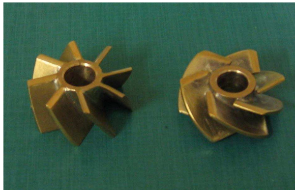
Figure 2.4: Swirlers with (a) 45^\circ vanes and (b) 60^\circ vanes.
